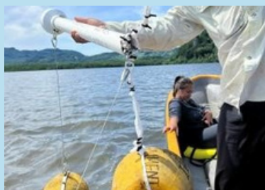
Deploying the turbidity sensor.
